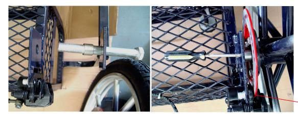
You can use a flat head screw driver to help install the inner axle sleeve. If the caliper pads fall out, you have to put them/it back, otherwise there will be no brake. And make sure the disk is inserted between the caliper pads.
