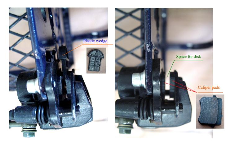
You may see a piece of plastic wedge inserted in between the brake pads for keeping the pads in place. Remove it and use a flat screw driver to push two pads into their caliper sockets. Make sure you have an open space to insert the brake disk into this space.
