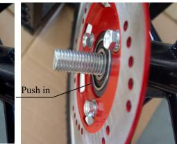
During the wheel-axle assembling, you need to make sure the ball bearing on wheel should be flashing to edge of disk, like right side picture shown. If ball bearing is stick out, you and push it in or use a mallet to tap it in. See left side pictures shown
